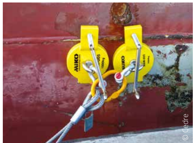
Magnetic anchoring system attached to vessel hull
